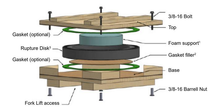
Disks rated with burst pressures less than 15 psig and without a vacuum support will be supplied with a foam membrane support
